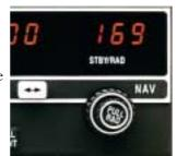
The lower-cost KX 155 system is virtually identical in appearance to the KX 165; however, it doesn't include the digital Radial readout feature. Also, the KX 155 requires an external VOR/LOC converter (usually included n the appropriate Bendix/King NAV indicator) while the KX 165 comes with a built-in VOR/LOC converter designed to interface directly with any ARINC standard CDI or HSI display.
